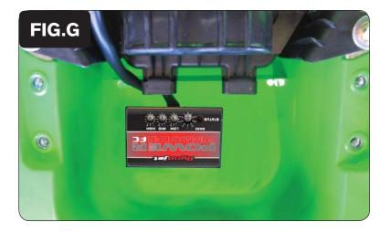
15 Using the supplied velcro, secure the PCFC to the rear fender as shown in Figure G.
