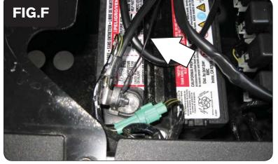
Attach the ground wire from the PCFC to the negative side of the battery as shown in Figure F.
