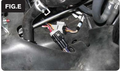
Attach the connectors from the PCFC to the stock wiring harness and throttle body harness as shown in Figure E.
