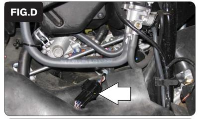
6 Unplug the stock wiring harness from the throttle bodies as shown in Figure D.
