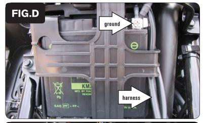
Attach the ground wire from the PCFC harness to the negative side of the battery as shown in Figure D.
