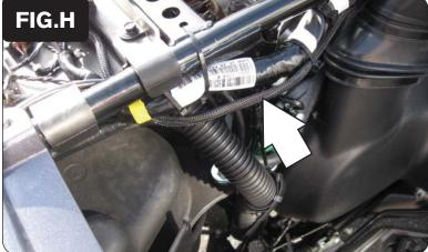
4 Route the PCFC harness under the plastic tray and down the right hand side of the ATV, following the stock wiring harness as shown in Figure H.
