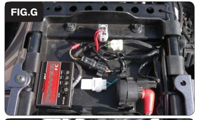
Using the supplied velcro, secure the PCFC to the tray under the seat as shown in Figure G.
