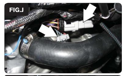
7 Attach the connectors from the PCFC wiring harness to the stock wiring harness and throttle body harness as shown in Figure J.
