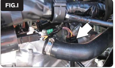
5 Locate the 6-pin BLACK connector on the front head, that comes from the throttle bodies as shown in Figure I.
