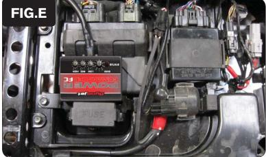
7 Using the supplied velcro, secure the PCFC to the top of the ECU as shown in Figure E.
