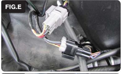
Attach the connectors from the PCFC harness to of the stock wiring harness as shown in Figure E.
