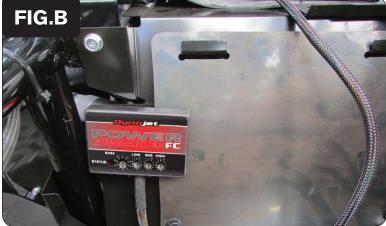
2 Using the supplied velcro, secure the PCFC to the panel below the drivers seat as shown in Figure B.
