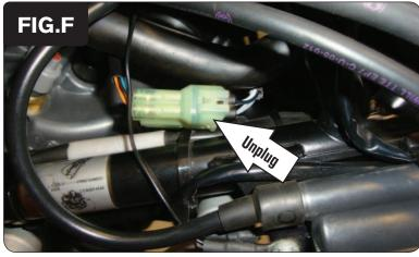
7 Locate and unplug the stock Throttle Position Sensor on the right side of the throttle body (Fig. D).
