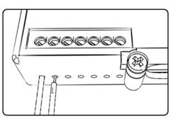
(Input 1 or 2) The PCV has the ability to hold 2 different base maps. You can switch on the fly between these two base maps when you hook up a switch to the MAP inputs. You can use any open/close type switch. The polarity of the wires is not important. When using the Autotune kit one position will hold a base map and the other position will let you activate the learning mode. When the switch is "CLOSED" Autotune will be activated. (Set to Switch Input #1 by default.)
