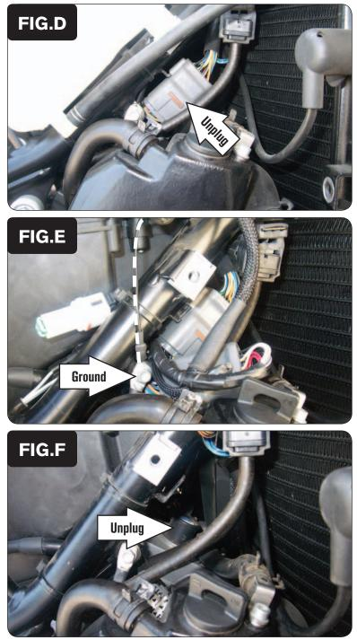
6 Locate the sub connector from the throttle bodies on the right side of the motorcycle. Unplug this connector.
