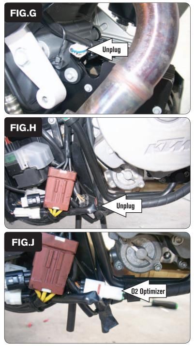
12 Locate the stock Crank Position Sensor connectors under the chin fairing at the front of the motorcycle (Fig. G).
