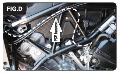
Route the PCV wiring harness inside of the frame rails and go towards the front of the engine (Fig. D).
