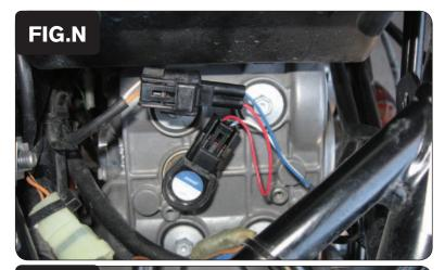
Plug the pair of PCV connectors with BLUE colored wires in-line of the Rear Ignition Coil and the stock wiring harness (Fig. N).
