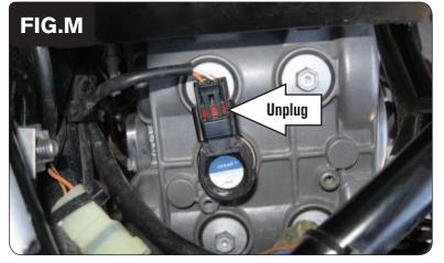
15 Unplug the stock wiring harness from the Rear Ignition Coil (Fig. M).
