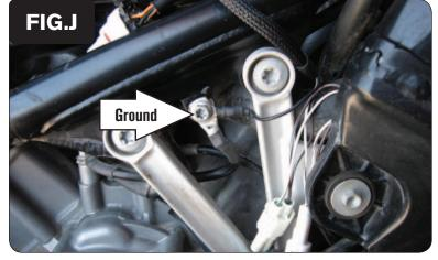
Secure the PCV ground wire with the small ring lug to the stock common ground location on the right side of the frame (Fig. J).
