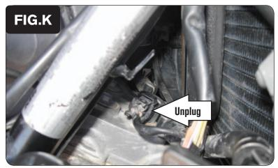
13 Unplug the stock wiring harness from the Front Ignition Coil (Fig. K).
