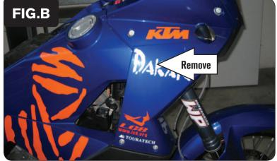
3 Remove the right and left hand side panels and fuel tanks (Fig. B).
