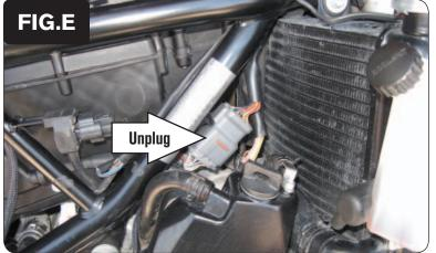
8 Unplug the stock throttle body sub-harness connector (Fig. E).
