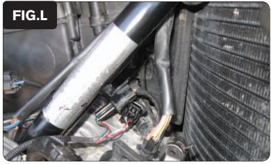
Plug the pair of PCV connectors with GREEN colored wires in-line of the Front Ignition Coil and the stock wiring harness (Fig. L).
