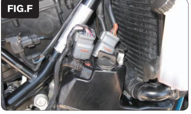
9 Plug the PCV main connectors in-line of the stock wiring harness (Fig. F).
