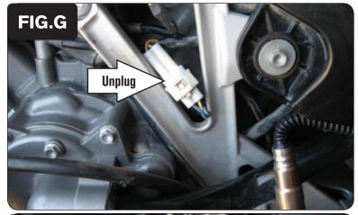
10 Locate the stock Crank Position Sensor connectors on the right side of the motorcycle. Unplug this connection (Fig. G).
