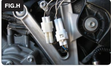
11 Plug the WHITE 2-pin connectors from the PCV wiring harness in-line of the stock Crank Position Sensor connectors (Fig. H).
