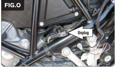
17 Locate the front cylinder O2 sensor connection.
