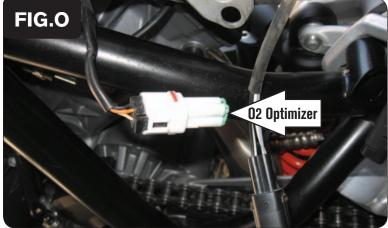
Plug the other supplied O2 Optimizer into the stock wiring harness in-place of the Rear O2 sensor (Fig. O).
