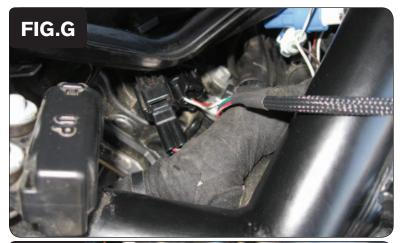
10 Plug the pair of PCV connectors the GREEN colored wires in-line of the Front Ignition Coil and the stock wiring harness (Fig. G).
