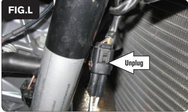
15 Unplug the stock Front O2 sensor from the main wiring harness (Fig. L).
