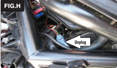
Locate the stock Crank Position Sensor connectors on the left side of the motorcycle. Unplug this connection (Fig. H).
