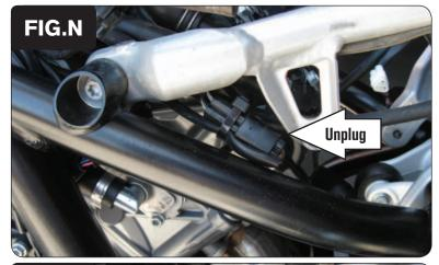
17 Unplug the stock Rear O2 sensor from the main wiring harness (Fig. N).
