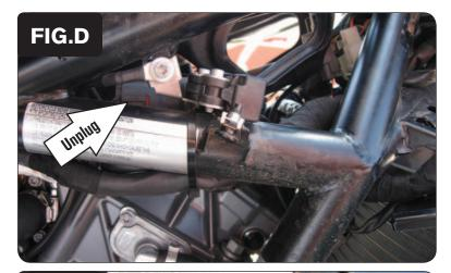
6 Locate the sub connector from the throttle bodies on the right side of the motorcycle. Unplug this connector (Fig. D).
