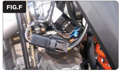
8 Plug the PCV in-line of the TPS and stock wiring harness (Fig. F).
