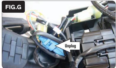
Unplug the stock Crank Position Sensor connectors (Fig. G). 9 This is the BLUE 2-pin connector in front of the ECU.
