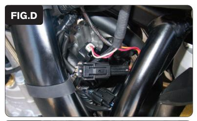
6 Plug the PCV in-line of the stock wiring harness and fuel injector (Fig. D).
