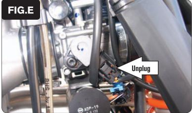
7 Unplug the stock wiring harness from the Throttle Position Sensor (Fig. E).
