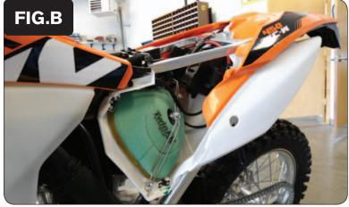
2 Remove the left side panel covering the air filter (Fig. B).
