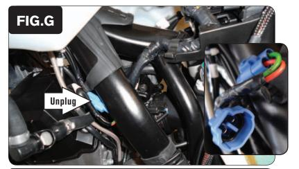
13 Locate and unplug the stock Crank Position Sensor connectors (Fig. G).
