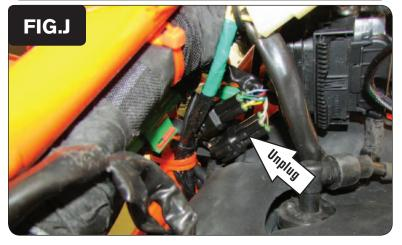
Unplug the stock crank position sensor connector (Fig. J).
