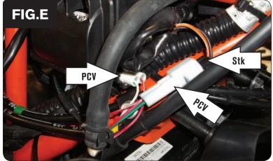
9 Plug the PCV in-line of the stock wiring harness and stock ignition coil (Fig. E)
