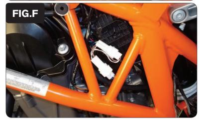
Plug the pair of WHITE 2-pin connectors from the PCV wiring harness in-line of the stock Crank Position Sensor connectors (Fig. F).
