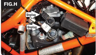
On the right side of the engine, locate and unplug the stock BLACK 2-pin connector from the inner coil stick and the stock WHITE 2-pin connector from the outer coil stick (Fig. H).
