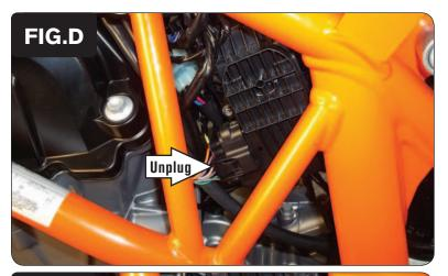
On the left side of the throttle body, locate and unplug the stock electrical connector from the Throttle Body Servo (Fig. D).
