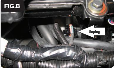
3 Unplug the stock wiring harness from the Throttle Position Sensor (Fig. B).
