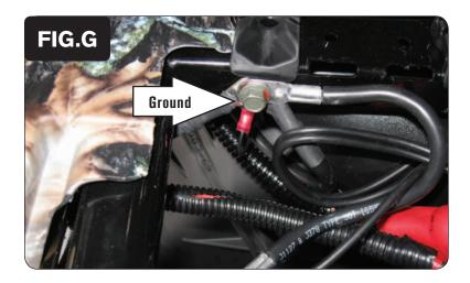
8 Attach the ground wire of the PCV to the ground bolt near the battery (Fig. G).
