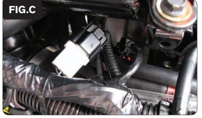
Plug the 3-pin connectors of the PCV in-line of the stock TPS and wiring harness (Fig. C).
