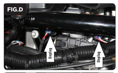
5 Unplug the stock wiring harness from each injector (Fig. D).
