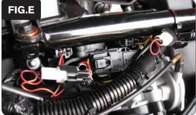
6 Plug the PCV in-line of the stock wiring harness and injectors (Fig. E).
