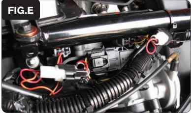
Plug the PCV in-line of the stock wiring harness and injectors (Fig. E).
