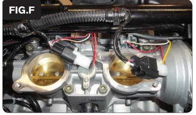
9 Plug the PCV in-line of the stock wiring harness and injectors (Fig. F).
