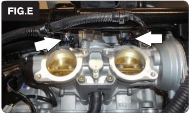
8 Unplug the stock wiring harness from both fuel injectors (Fig. E).
