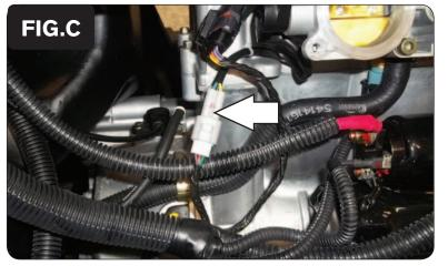
6 Unplug the stock wiring harness from the Throttle Position Sensor.
