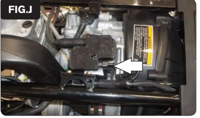
THE FOLLOWING STEPS WERE DONE ON A SCRAMBLER. FOR THE SPORTSMAN THE IGNITION COIL IS ON THE RIGHT SIDE OF THE AIRBOX NEAR THE SHIFT LEVER.
