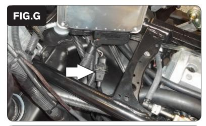
10 Locate the stock Crank Position Sensor connector and unplug it (Fig. G).
