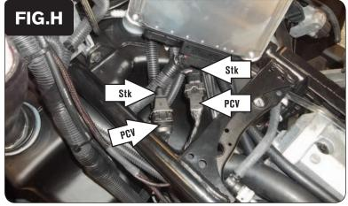
11 Plug the PCV harness in-line of the stock CPS and wiring harness (Fig. H).
