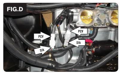
7 Plug the PCV harness in-line of the stock TPS and wiring harness (Fig. D).
