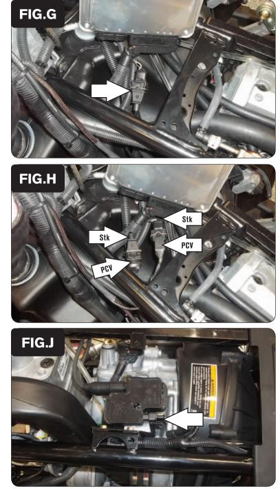
10 Locate the stock Crank Position Sensor connector and unplug it (Fig. G). This is a BLACK 3-pin connector located near the ECM, underneath the airbox.
