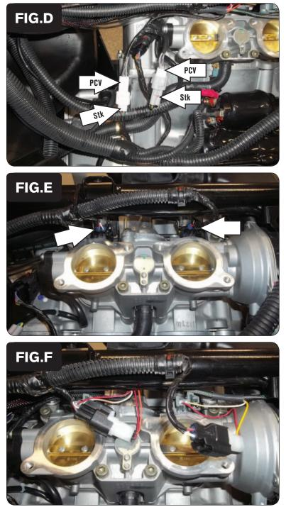
7 Plug the PCV harness in-line of the stock TPS and wiring harness (Fig. D).
