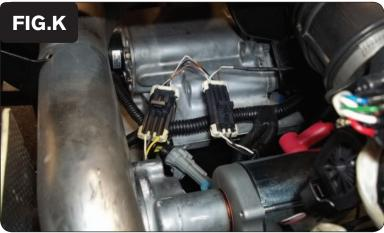
14 Locate and unplug the stock Crank Position Sensor connectors (Fig. J). This is the BLACK connector pair; not the GREY pair.
