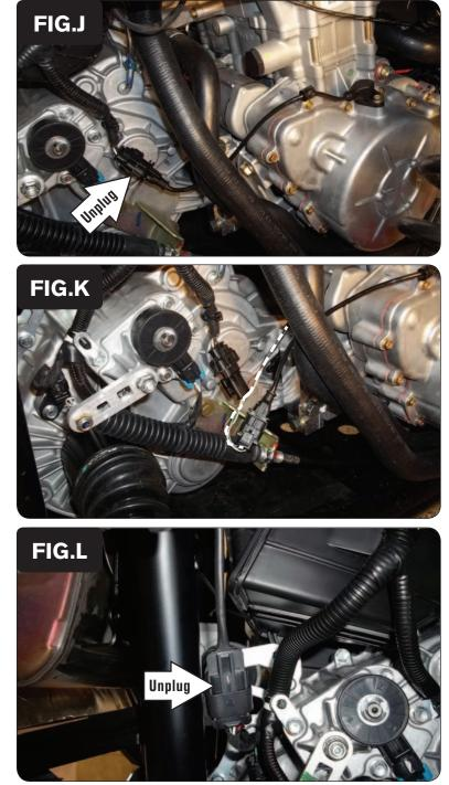
20 Locate and unplug the stock pair of connectors for the engine's Crank Position Sensor (Fig. J).
