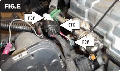
Plug the pair of PCV wiring harness leads with ORANGE colored wires in-line of the Fuel Injector and the stock wiring harness (Fig. E).
