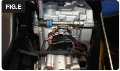
Plug the PCV wiring harness in-line of the Fuel Injector and the stock wiring harness (Fig. E).
