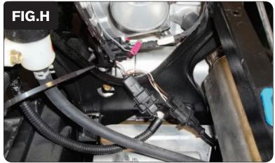
11 Plug the PCV wiring harness in-line of the stock Crank Position Sensor connectors (Fig. H).
