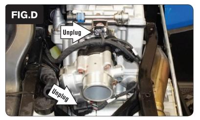
6 Unplug the Fuel Injector and the Throttle Body Servo connector (Fig. D).
