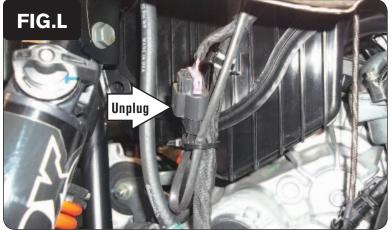
19 Unplug the stock O2 sensor connectors (Fig. L).
