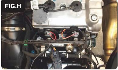
Plug the PCV wiring harness in-line of the Fuel Injectors and the stock wiring harness (Fig. H).
