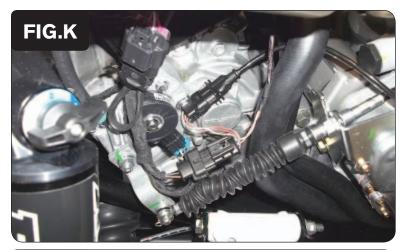
18 Plug the pair of PCV connectors with BROWN colored wires in-line of the stock Crank Position Sensor connectors (Fig. K).
