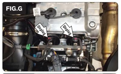
14 Unplug both of the Fuel Injectors. These are located at the top of the throttle bodies (Fig. G).
