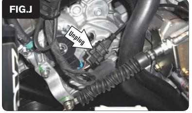
17 Unplug the stock Crank Position Sensor connectors (Fig. J).
