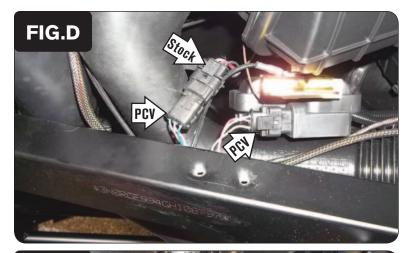
Plug the pair of PCV wiring harness connectors with BLUE and GREEN colored wires in-line of the Ignition Coil and the stock wiring harness (Fig. D).
