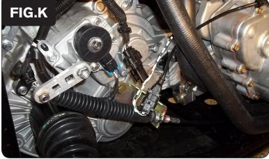
20 Locate and unplug the stock pair of connectors for the engine's Crank Position Sensor (Fig. J).
