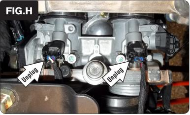
Locate and unplug the stock wiring harness from both of the fuel injectors (Fig. H).
