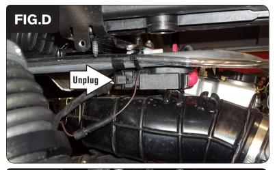
Locate and unplug the stock electrical connector from the vehicle's ignition coil (Fig. D).
