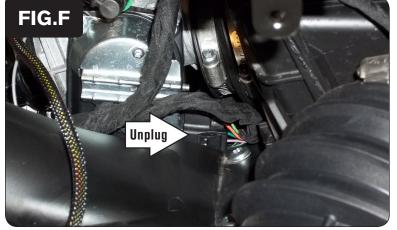
Unplug the electrical connector for the throttle body servo on the left side of the throttle bodies (Fig. F).
