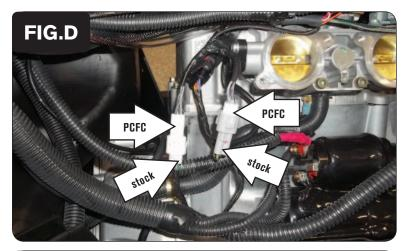
7 Attach the connectors from the PCFC to the stock TPS and wiring harness as shown in Figure D.
