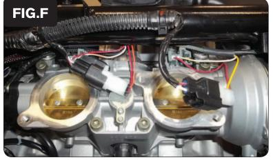
9 Attach the connectors from the PCFC to the injectors and stock wiring harness as shown in Figure F.
