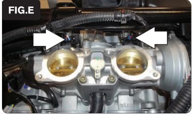
8 Unplug the stock wiring harness from each injector as shown in Figure E.
