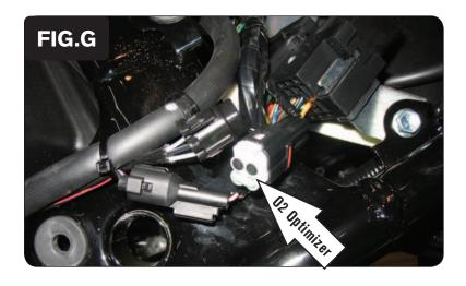
12 Locate the stock O2 sensor connection.
