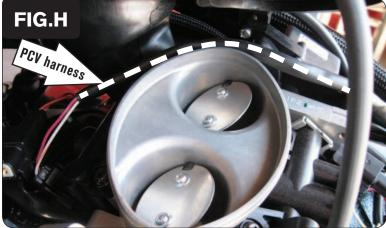
11 Loosen the clamp that holds the intake duct to the throttle body. Lift up on the intake duct so the PCV harness can be routed underneath this duct and in front of the throttle body (Fig. H).
