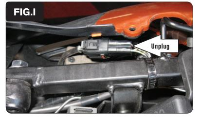
17 Locate the wiring harness connectors for the bike's stock O2 sensor. These connectors are on the right side of the bike under the seat and directly above the rear brake fluid reservoir. Unplug the connectors for the stock O2 sensor (Fig. I).
