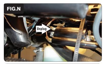
20 Locate and unplug only the stock GREY wire from the right side Ignition Coil (Fig. N).
