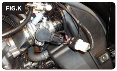
Plug the pair of 3-pin connectors of the PCV wiring harness in-line of the bike's TPS and the stock wiring harness (Fig. K).
