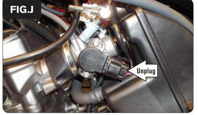
Locate and unplug the stock wiring harness from the bike's Throttle Position Sensor on the left side of the throttle bodies (Fig. J).
