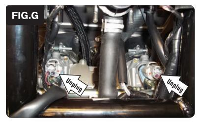
Locate and unplug the stock connectors from both Fuel Injectors at the top of the throttle bodies (Fig. G).
