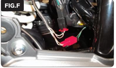
Plug the pair of RED 2-pin PCV connectors with BROWN colored wires in-line of the stock Crank Position Sensor connectors (Fig. F).
