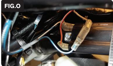
Plug the pair of PCV leads with BLUE and WHITE/BLUE wires in-line of the stock GREY wire and the right Ignition Coil (Fig. O).
