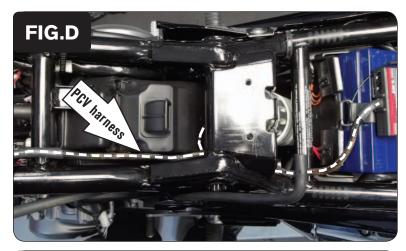
9 Route the PCV wiring harness forward along the left side frame rail going under the frame cross-member for the rear shock (Fig. D).
