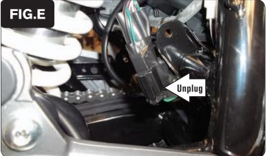
Locate and unplug the stock connectors for the bike's Crank Position Sensor (Fig. E).
