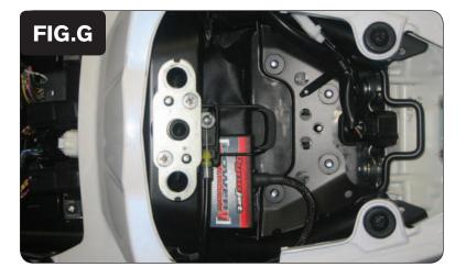
13 Install the PCV in the tail section. Use the supplied Velcro to secure the unit in the tail (Fig. G).
