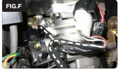
Plug the connectors from the PCV in-line of the stock wiring harness and the TPS (Fig. F).
