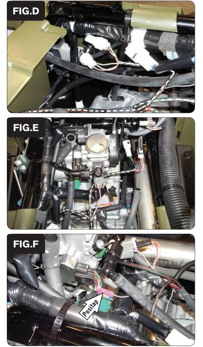
9 Plug the pair of PCV connectors with BROWN colored wires in-line with the stock Crank Position Sensor connectors (Fig. D).
