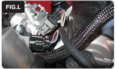
9 Attach the PCFC connectors to the stock wiring harness and the injectors as shown in Figure J.
