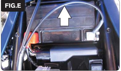
11 Attach the ground wire from the PCFC to the negative side of the battery as shown in Figure E.
