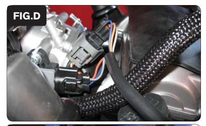
10 Attach the 3-pin connectors from the PCFC to the TPS and stock wiring harness as shown in Figure D.
