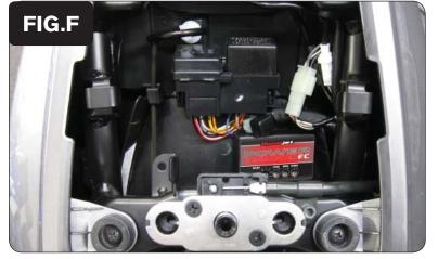
12 Using the supplied velcro, secure the PCFC in the tail section as shown in Figure F.
