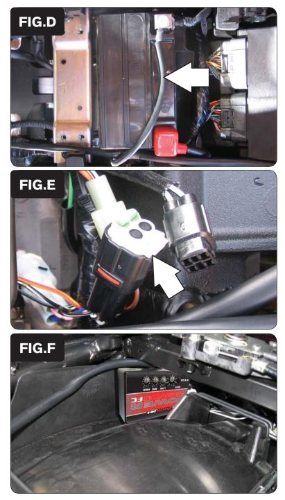
8 Attach the ground wire from the PCFC to the negative side of the battery as shown in Figure D.
