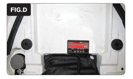
Using the supplied velcro, secure the PCFC to the rear fender as shown in Figure D.
