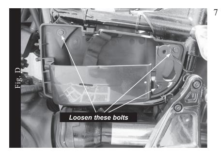
Loosen the bolts holding the plastic tray on the left side of the bike (under the left side cover) (Fig. D).
