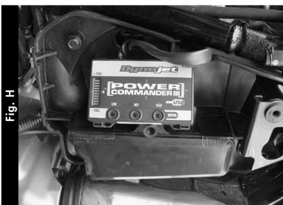
11 Install the PCIII under the left hand side cover. You can use the supplied velcro to attach it in place.
