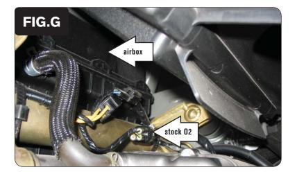
11 Locate the stock O2 sensor where it connects to the main wiring harness as shown in Figure G.
