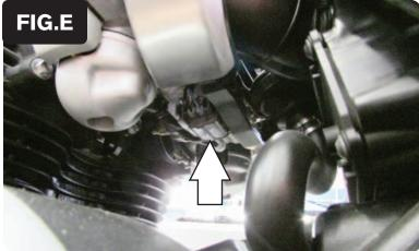
8 Unplug the stock Throttle Position Sensor connector(Fig. E).
