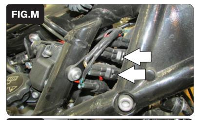
16 Unplug the stock O2 sensor connectors (Fig. M).
