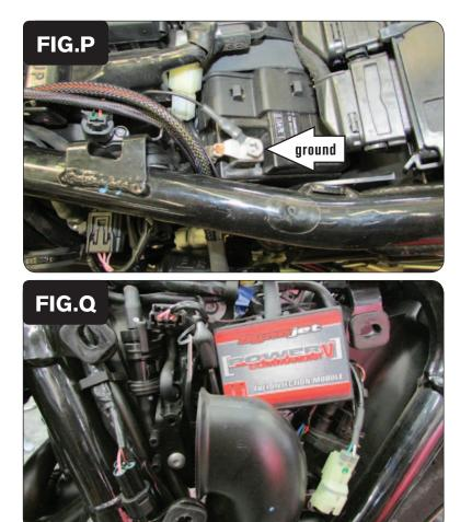
19 Attach the ground wire from the PCV to the negative (-) side of the battery (Fig. P).
