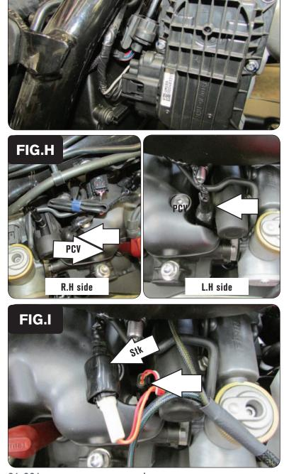
10 Plug the TPS connectors from the PCV in-line of the stock throttle body and wiring harness (Fig. G).
