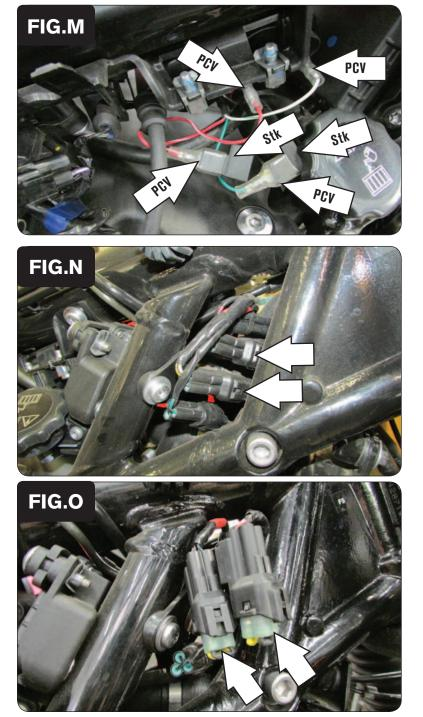
Plug the PCV in-line of the stock wiring harness and ignition coil (Fig. M).
