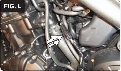
13 Unplug the stock O2 sensor (Fig. L).
