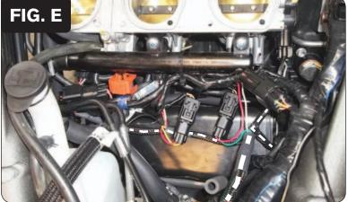
Plug the PCV wiring harness in-line of each Fuel Injector and the stock wiring harness (Fig. E).
