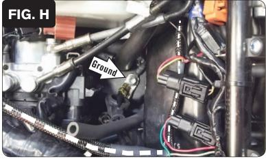
Secure the PCV ground wire with the small ring terminal and the stock ground wires to the crank case using the stock common ground bolt (Fig. H).
