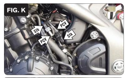
12 Plug the PCV wiring harness in-line of the stock Crank Position Sensor connectors (Fig. K).
