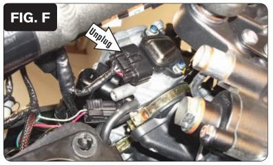
8 Unplug the Throttle Position Sensor (Fig. F).
