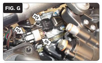
9 Plug the PCV wiring harness in-line of the Throttle Position Sensor and the stock wiring harness (Fig. G).
