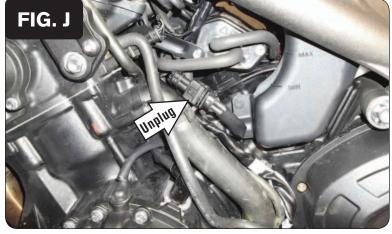
11 Unplug the stock Crank Position Sensor connectors (Fig. J).
