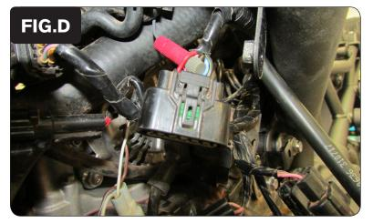
Unplug the stock wiring harness from the bike's Throttle Position Sensor on the left hand side of the throttle bodies.
