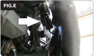
7 Plug the stock TPS connector back onto the TPS (Fig. E).
