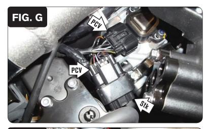
10 Plug the PCV wiring harness in-line of the Throttle Position Sensor and the stock wiring harness (Fig. G).
