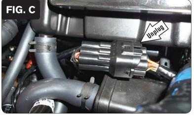
5 Unplug the stock BLACK 6-pin connector pair located just behind the airbox (Fig. C).
