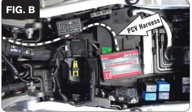
3 Secure the PCV module in the tail section under the seat with the supplied Velcro (Fig. B).
