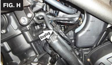
11 Unplug the stock Crank Position Sensor connectors (Fig. H).
