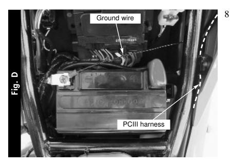
Route the ground wire from the PCIII under the frame and attach to the negative side of the battery (Fig. D).
