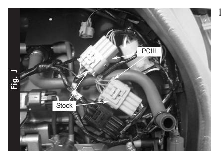
11. Plug the other connectors from the PCIII in-line of the stock TPS connectors (Fig. J).
