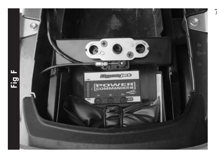
Install the PCIII in the tail section using the supplied velcro. Make sure to clean both surfraces before attaching unit (Fig. F).
