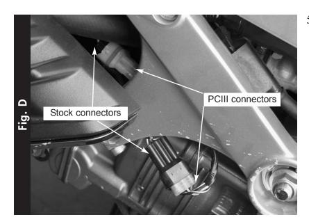
5 Plug the PCIII in-line of these connectors (Fig. D).
