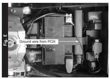
Attach the ground wire from the PCIII to the negative side of the battery (Fig. E).
