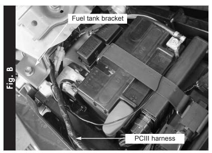
Route the wires from the PCIII under the fuel tank bracket and go towards the front of the bike on the left hand side of the engine (Fig. B)
