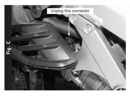
4 Unplug the connector from the throttle bodies (Fig. C). This connector is located on the L.H side of the engine behind the frame rail. It is black in color.
