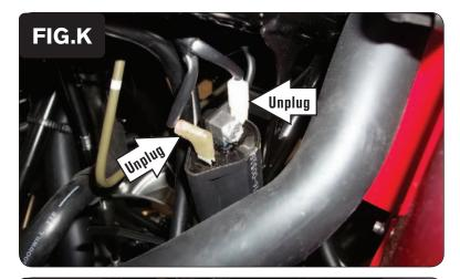
Locate the Ignition Coil on the right side of the quad forward of the engine and unplug the 2 stock coil wires (Fig. K).
