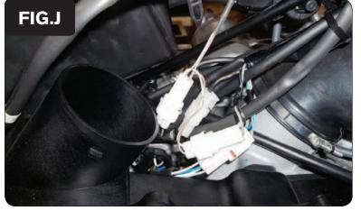
Plug the WHITE 2-pin connectors from the PCV wiring harness in-line of the stock Crank Position Sensor connectors (Fig. J).
