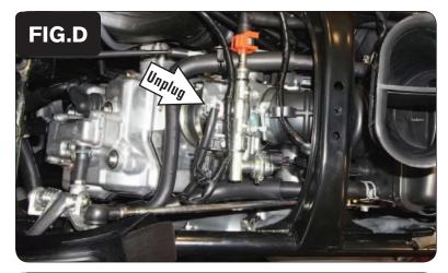
8 Unplug the stock wiring harness from the Fuel Injector (Fig. D).
