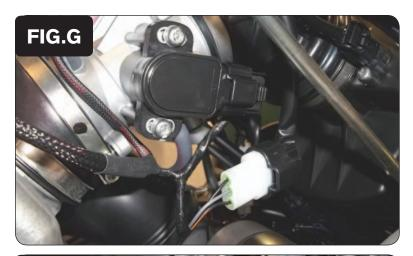
Plug the pair of 3-pin connectors of the PCV in-line of the Throttle Position Sensor and the stock wiring harness (Fig. G).
