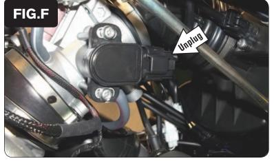
Locate and unplug the stock wiring harness from the Throttle Position Sensor (Fig. F).
