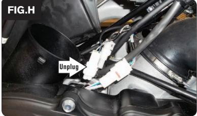
Locate and unplug the stock connectors from the Crank Position Sensor (Fig. H).
