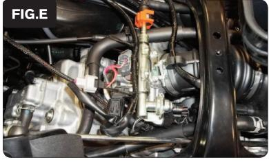
9 Plug the pair of PCV connectors with ORANGE colored wires in-line of the stock wiring harness and the Fuel Injector (Fig. E).
