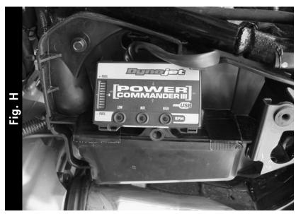
Install the PCIII under the left hand side cover (Fig. H).
