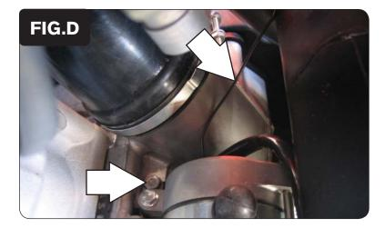
8 Attach the ground wire from the PCFC to the main engine ground as shown in Figure D.
