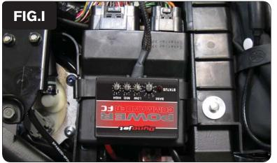
17 Using the supplied velcro, secure the PCFC on top of the ECU as shown in Figure I.
