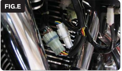
8 Attach the PCFC connectors to the throttle bodies and stock wiring harness as shown in Figure E.
