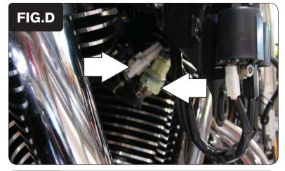
7 Unplug the white 3-pin connector and the clear 6-pin connector as shown in Figure D.
