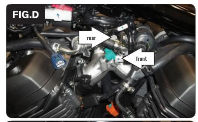
9 Unplug the stock wiring harness from the front and rear cylinder fuel injectors.
