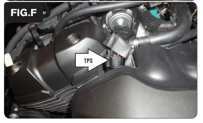
12 Unplug the Throttle Position Sensor (TPS) connector.
