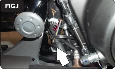
15 Attach the connectors from the PCFC to the stock O2 sensor and wiring harness.
