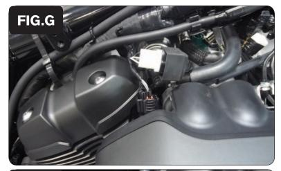
13 Attach the connectors from the PCFC to the TPS and stock wiring harness.
