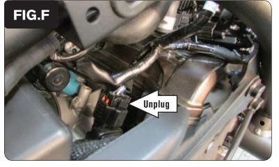
9 Unplug the stock wiring harness from the Throttle Position Sensor located on the right side of the throttle bodies (Fig. F).
