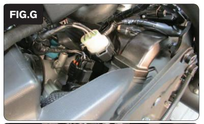
10 Plug the PCFC wiring harness in-line of the TPS and the stock wiring harness (Fig. G).
