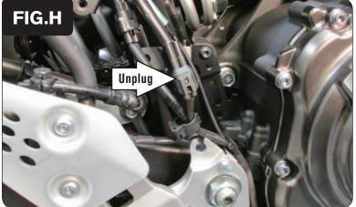
Just above the right footpeg, locate and unplug the stock connector for the bike's O2 sensor (Fig. H).
