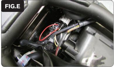
Plug the PCFC wiring harness in-line of the Fuel Injectors and the stock wiring harness (Fig. E).
